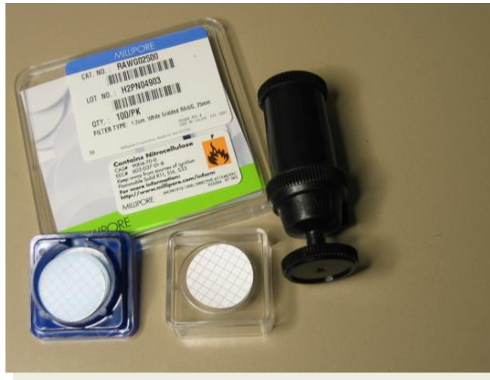
Fig. 1 Exploded view of a personal sampling head
